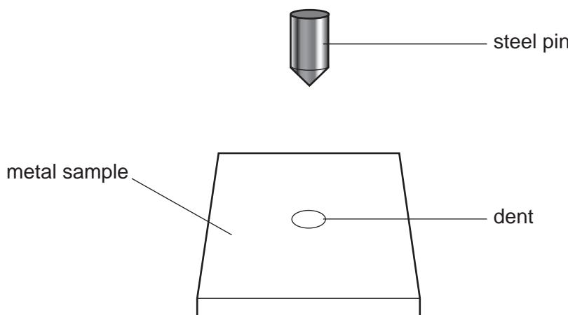
The depth of the dent produced is measured on a scale of 0 to 100.
