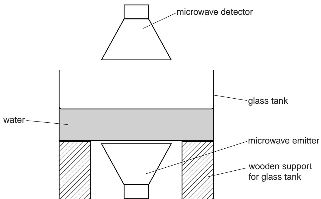
Anita and Vijay measure the depth of the water in the tank and the intensity of the microwave signal received by the detector.
