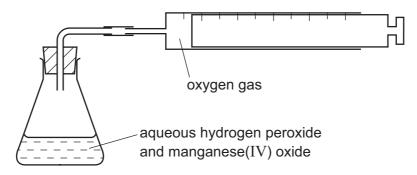
40 cm<sup>3</sup> of aqueous hydrogen peroxide was put in the flask and 0.1 g of small lumps of manganese(IV) oxide was added. The volume of oxygen collected was measured every 30 seconds. The results were plotted to give the graph shown below.
