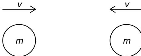
The spheres have a head-on elastic collision.
