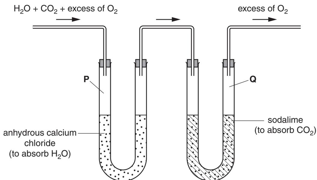
The increases in mass of the collecting vessels **P** and **Q** of the apparatus are  $M_P$  and  $M_Q$ , respectively.
