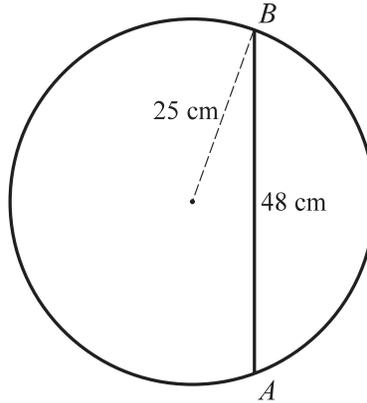
A frame consists of a uniform circular ring of radius 25 cm and mass 1.5 kg, and a uniform rod of length 48 cm and mass 0.6 kg. The ends  $A$  and  $B$  of the rod are attached to points on the circumference of the ring, as shown in the diagram. Find the distance of the centre of mass of the frame from the centre of the ring. [4]
