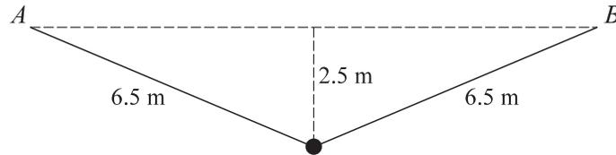
A light elastic string has natural length 10 m and modulus of elasticity 130 N. The ends of the string are attached to fixed points  $A$  and  $B$ , which are at the same horizontal level. A small stone is attached to the mid-point of the string and hangs in equilibrium at a point 2.5 m below  $AB$ , as shown in the diagram. With the stone in this position the length of the string is 13 m.
