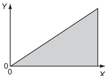
The shaded area represents the total strain energy stored in stretching the wire.
