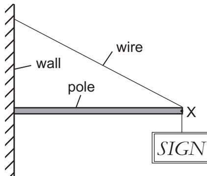
The force exerted by the pole at point X is  $F$ , and the tension in the wire is 40 N.
