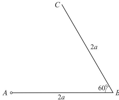
Two uniform rods  $AB$  and  $BC$ , each of length  $2a$  and mass  $m$ , are rigidly joined at  $B$  so that angle  $ABC = 60^\circ$  (see diagram). The system is free to rotate in a vertical plane about a horizontal axis through  $A$ . Show that the moment of inertia of the system about this axis is  $\frac{14}{3}ma^2$ . [3]
