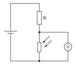
What happens to the voltmeter reading, and why does it happen, when the intensity of light on the LDR increases?
