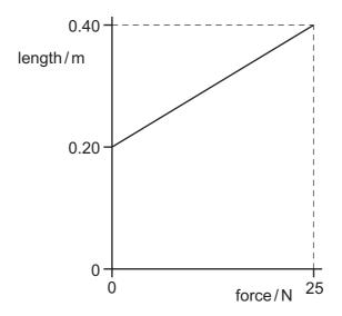
What is the maximum strain energy in this deformed rubber cord?
