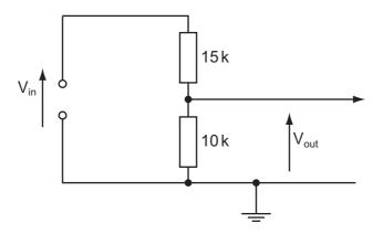
$V_{out}$  is equal to 4.8 V.
