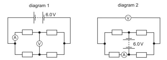
The resistors and meters are reconnected to the supply as shown in diagram 2.
