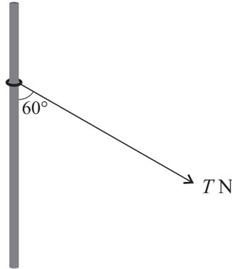
A ring of mass  $4 \text{ kg}$  is threaded on a fixed rough vertical rod. A light string is attached to the ring, and is pulled with a force of magnitude  $T \text{ N}$  acting at an angle of  $60^\circ$  to the downward vertical (see diagram). The ring is in equilibrium.
