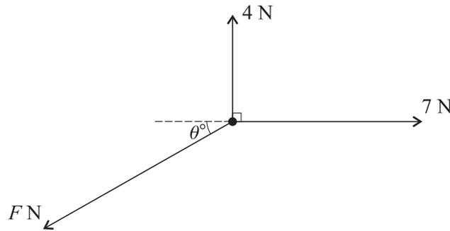
A particle is in equilibrium on a smooth horizontal table when acted on by the three horizontal forces shown in the diagram.
