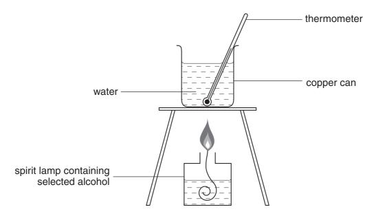
[4.2J of heat energy raise the temperature of 1 cm<sup>3</sup> (1 g) of water by 1 °C.]
