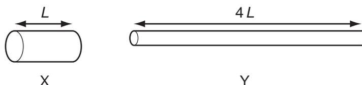
What is the ratio  $\frac{\text{resistance of wire Y}}{\text{resistance of wire X}}$ ?
