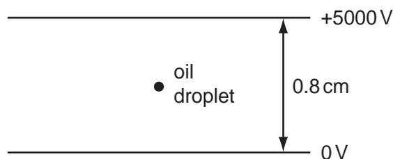
What is the magnitude and direction of the electrostatic force on the oil droplet?
