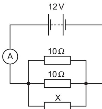
The battery has e.m.f. 12V and negligible internal resistance. The ammeter reading is 3.2A.
