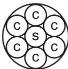
1.0 km of one of the copper wires has a resistance of  $10 \Omega$  and 1.0 km of the steel core has a resistance of  $100 \Omega$ .
