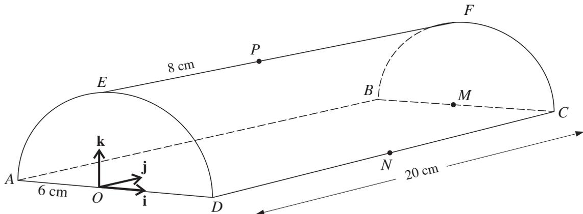
The diagram shows a semicircular prism with a horizontal rectangular base  $ABCD$ . The vertical ends  $AED$  and  $BFC$  are semicircles of radius 6 cm. The length of the prism is 20 cm. The mid-point of  $AD$  is the origin  $O$ , the mid-point of  $BC$  is  $M$  and the mid-point of  $DC$  is  $N$ . The points  $E$  and  $F$  are the highest points of the semicircular ends of the prism. The point  $P$  lies on  $EF$  such that  $EP = 8$  cm.
