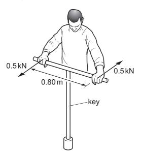
What is the torque produced by the couple on the key?
