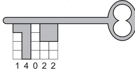
The columns of the key can be any integer length from 0 to 4 – except that the extreme case of **0 0 0 0 0** is not permissible because it would not turn any lock.
