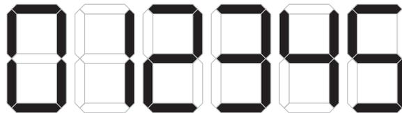
Create a blank seven-segment display, 60 pixels wide and 110 pixels high, using a 1-point grey (150,150,150 RGB) outline.
