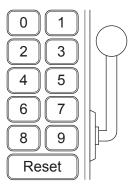
The box is opened by pressing Reset, entering a code and then pulling a lever. The code must have between one and five different digits (inclusive).
